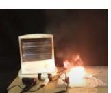
**Overloading your current can** The standard capacity of a power cause fires! Electrical Consumption 3400W > Set Capacity 1500W = Overloading!
