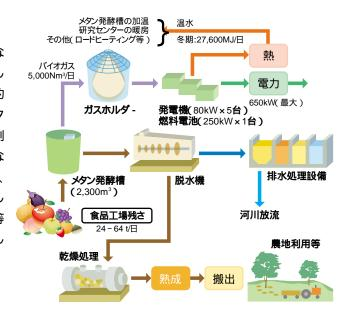
A biogas power generation plant capable of supplying a controllable source of power constitutes a system that works by sorting and accepting food material rejected by food factories, among others, and producing gas through a methane fermentation process in order to furnish gas to engine-based power generators and fuel cells as a means of generating a stable supply of electricity.
